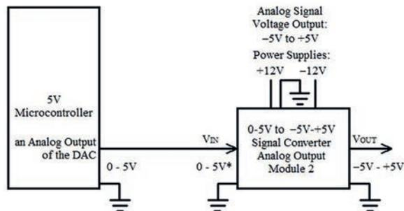
Figure 6: Analogue output module 2's connections to a 5V microcontroller
