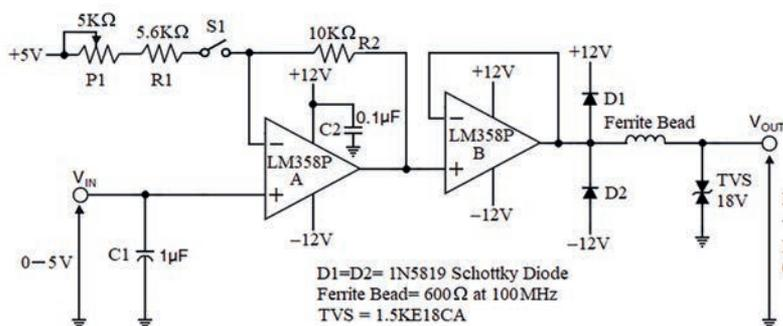
Figure 1: Circuit diagram of the analogue output module 1 for a 0-5V to -5V - +5V signal converter
