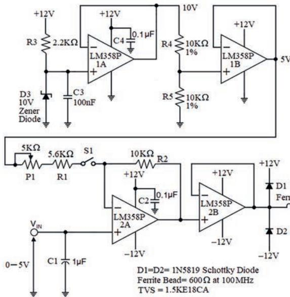
Figure 5: Circuit diagram of the analogue output module 2 for a 0-5V to -5V - +5V signal converter
