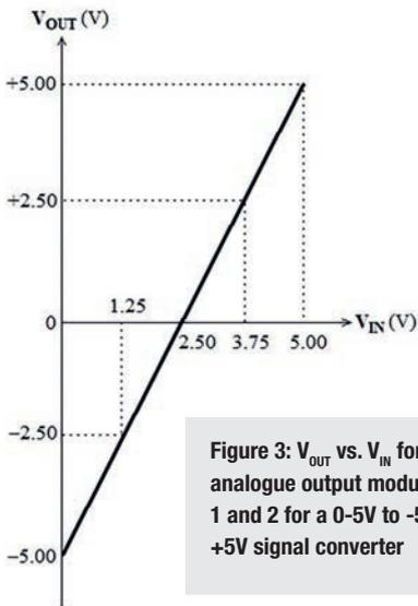
Figure 3:  $V_{out}$  vs.  $V_{in}$  for analogue output modules 1 and 2 for a 0-5V to -5V - +5V signal converter
