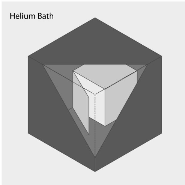
*Figure 3: Schematic representation of a thought experiment. A large outer cavity acts as an ideal blackbody (emissivity = 1, reflectivity = 0) and is initially immersed in a helium bath at 4K. Within this cavity, a perfectly reflecting cavity (emissivity = 0, reflectivity = 1) rests of the floor with one of its sides initially remaining open*
