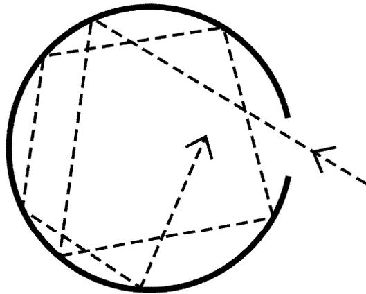
*Figure 1: Schematic representation of radiation incident upon a spherical cavity*
